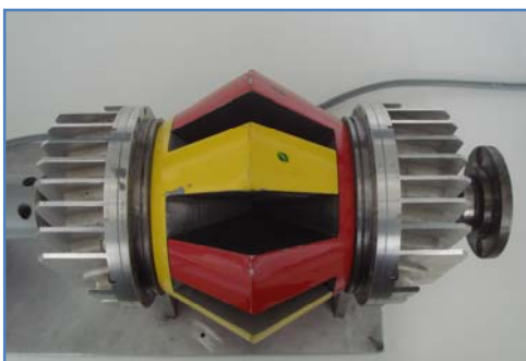
Fig. 7: View into the interior of a Schukey engine. What can be seen are the two rotor-blade crosses (red and yellow). The two gear units are at the right and left ends. Each gear unit drives its respective rotor.
